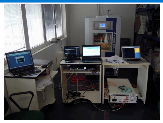
Managed to ensure error-free operation in -15C/+75C environment, and in presence of EMI fields of up to 180V/m. Yeah!
