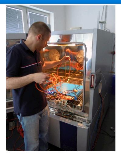
Managed to ensure error-free operation in -15C/+75C environment, and in presence of EMI fields of up to 180V/m. Yeah!
